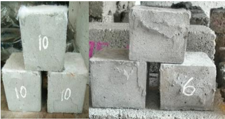
Fig. 3 Typical failure mode of ECC cubes after compressive test
