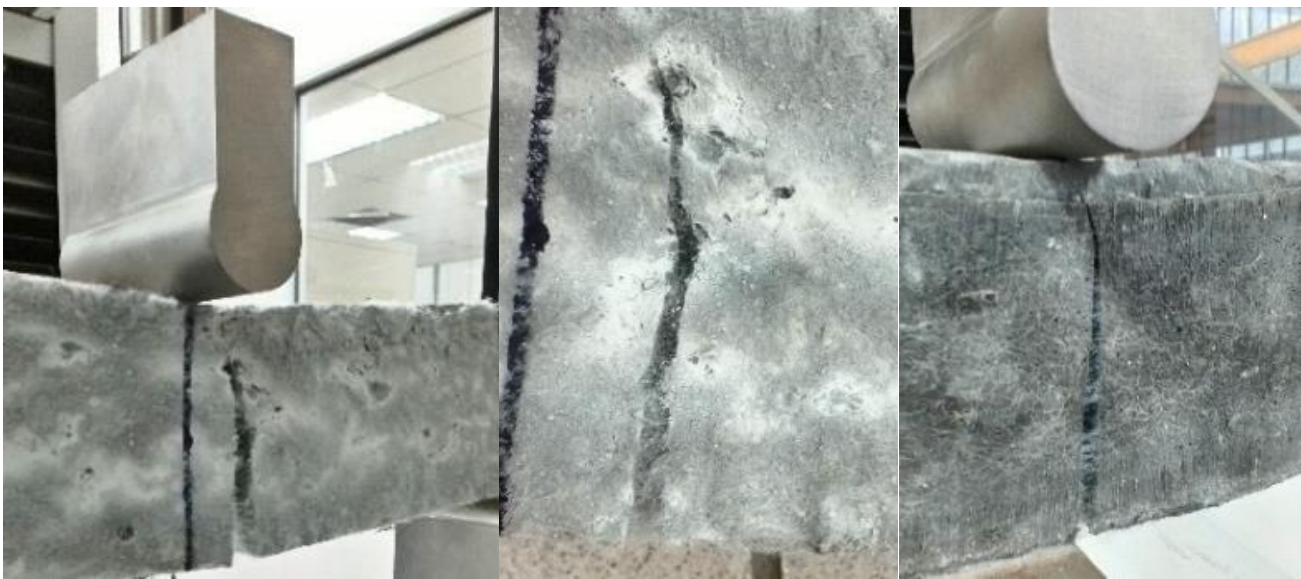
Fig. 5 Typical behavior of ECC specimens under flexural test
