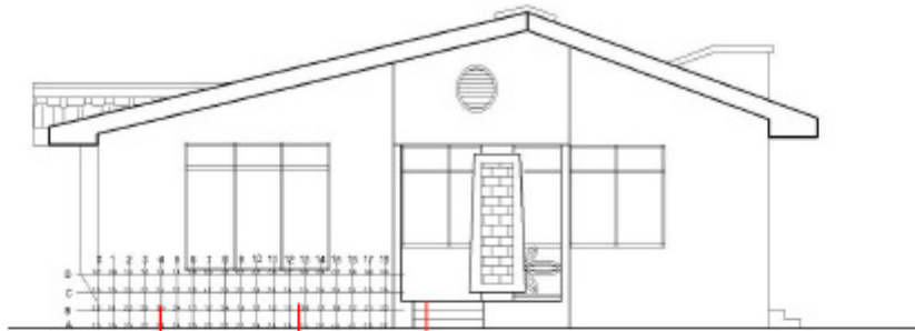
Figure 6a. Moisture contents on walls in the western orientation
