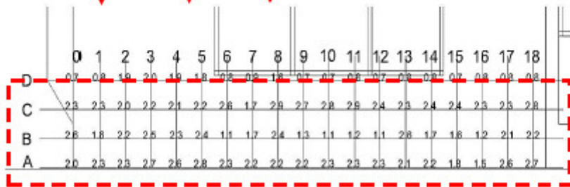
Figure 6b. Enlarged 300mmx300mm grids showing moisture contents on walls in western orientation
