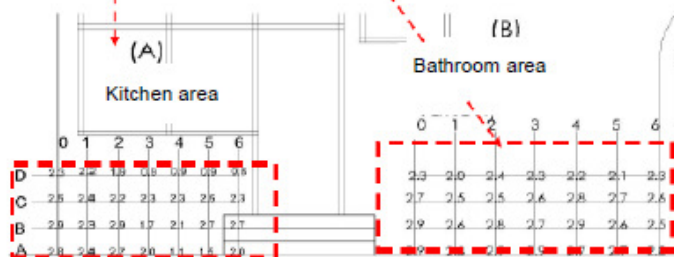
Figure 7c. Moisture content distribution on walls of kitchen and bathroom in the southern orientation
