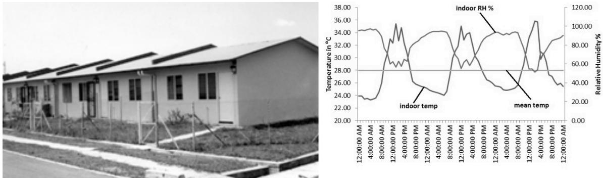
Figure 2: Typical low cost housing indoor climate in Kuching Sarawak. Left: Typical low cost house for low income earners in Sarawak (HDC Sarawak, 2015). Right: Typical low income house indoor climate measure from 30/10/2014 to 1/11/2014
