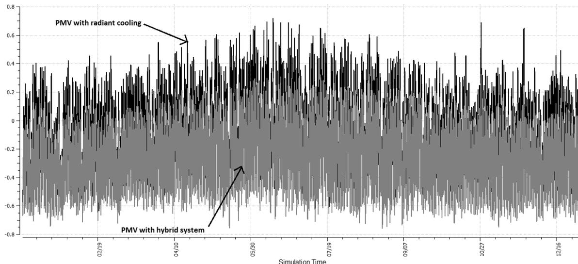
Figure 12: PMV comparison of radiant system only model and hybrid system
