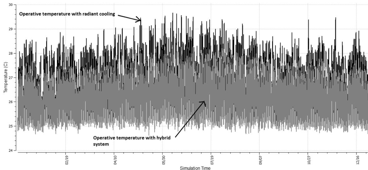
Figure 10: Annual operative temperature comparison for radiant system only model and hybrid system
