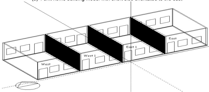
(b) 4 units home building with separate thermal zone for each unit
