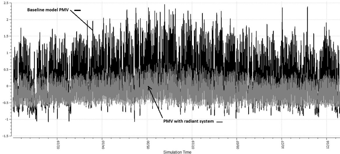
Figure 11: PMV comparison of baseline model and the radiant system model.
