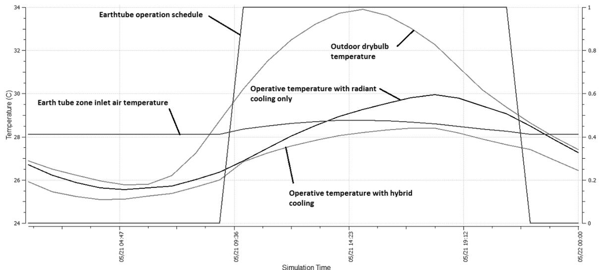
Figure 14: East unit zone operative temperature further reduction by hybrid system
