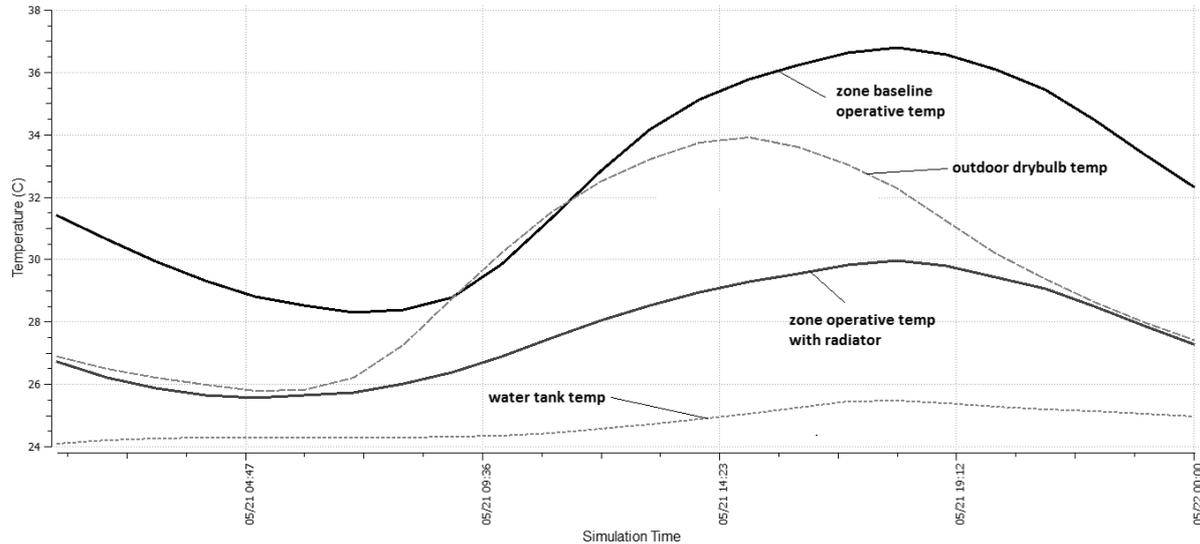
Figure 13: Baseline east unit zone operative temperature reduction by radiant cooling system with renewable water source
