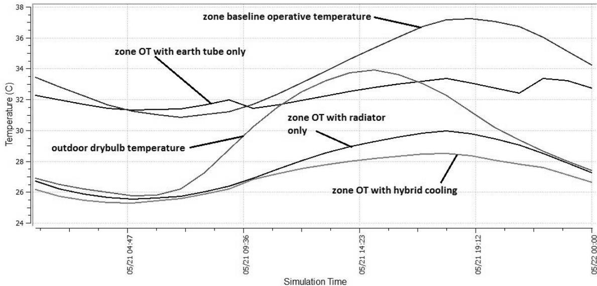
Figure 15: East unit zone operative temperature with the application of earth tube system, radiator system and hybrid system respectively
