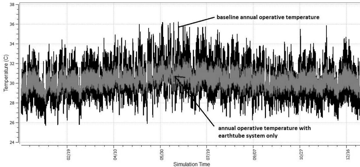
Figure 9: Annual operative temperature comparison of baseline model with earth tube cooling system only
