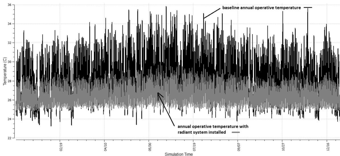
Figure 8: Annual operative temperature comparison of baseline model with radiant cooling system only
