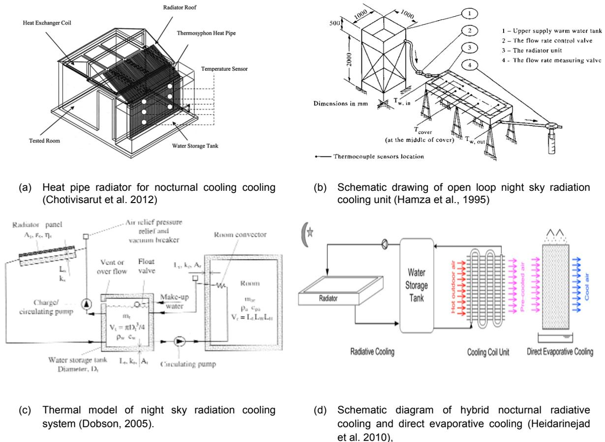
Figure 1: Example of a few prototypes which uses night cooling in its operation
