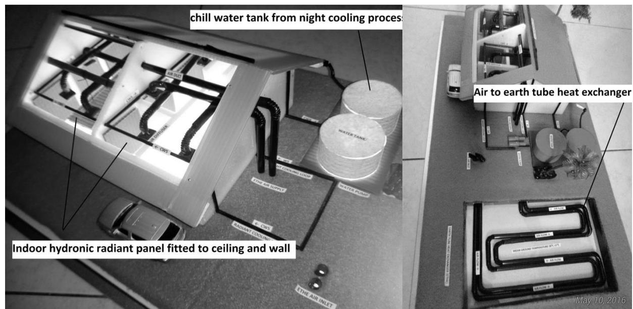
Figure 3: Concept model of the hybrid system which uses night sky and cool ground as heat sink to cool the building
