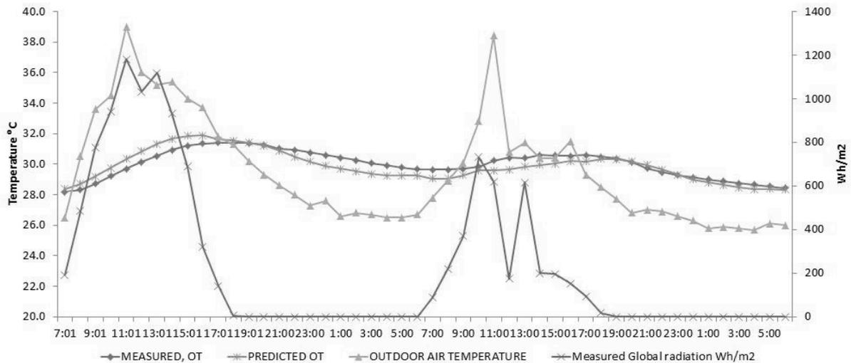
Figure 7: Comparison of predicted operative temperature of thermal zone 6 by Energy Plus and measured on site
