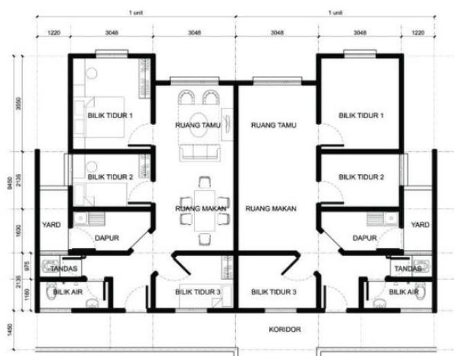
Figure 2: Standard PPR Housing Unit Floor Plan
