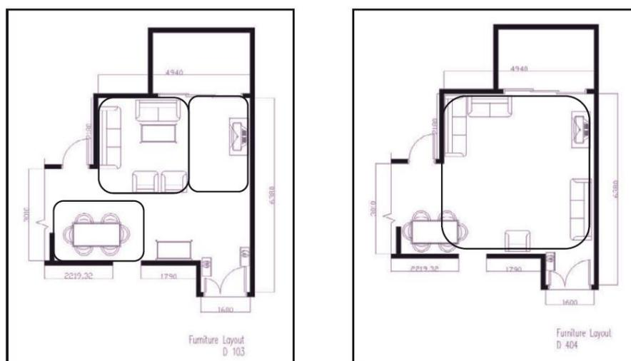
Figure 3: Type (A) Clustered furniture arrangement & Type (B) Centralised furniture arrangements
