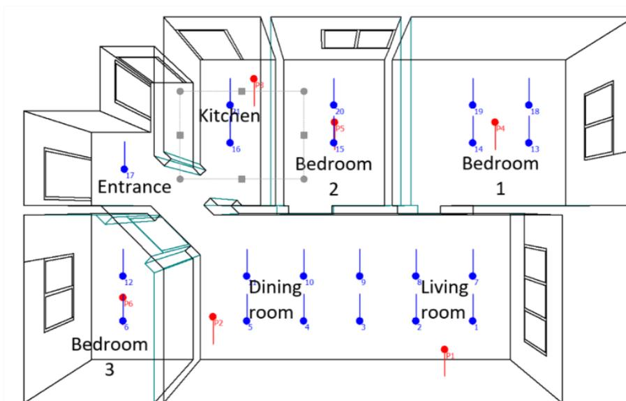
Figure 6: The locations of sources and receivers in the ODEON model.
