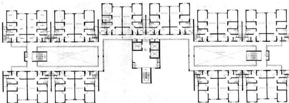
Figure 1: Typical Level Layout Plan for 18-storey PPR Low-cost Flat
