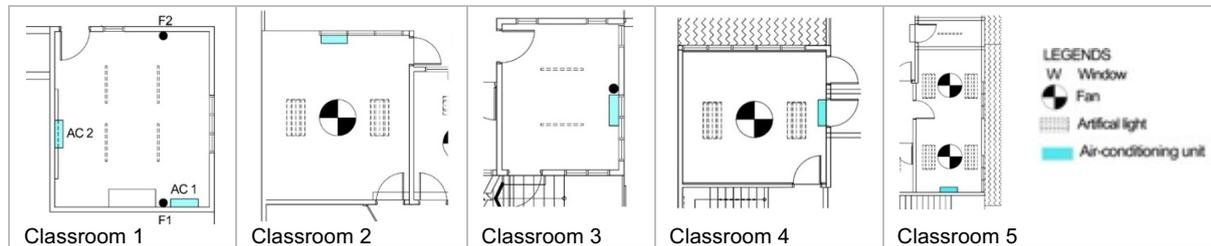
Figure 10: Location of Air conditioning unit and fan in classroom 1, 2, 3, 4 and 5.
