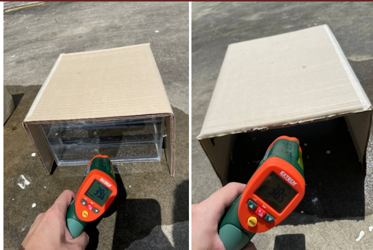
Figure 6: a) Outdoor Surface Temperature Test, b) Indoor Surface Temperature Test
