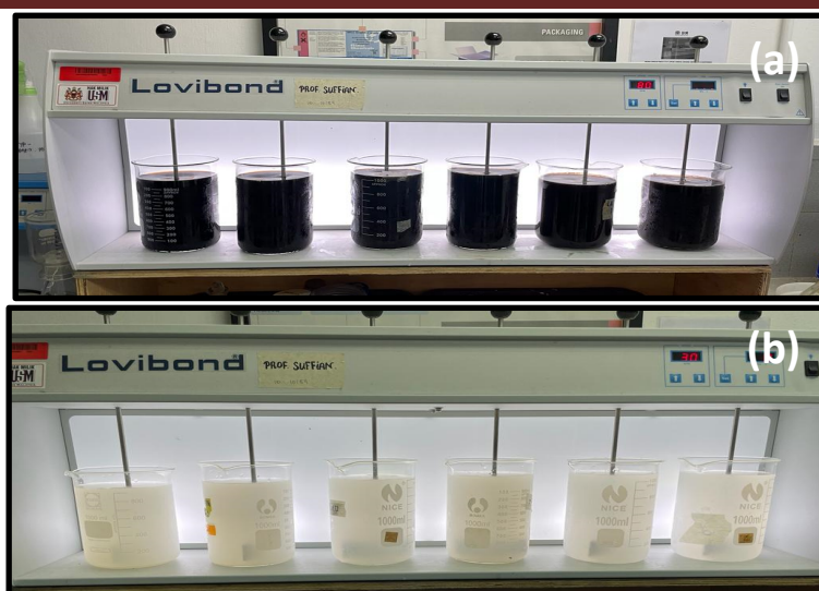
Rajah 2: Persediaan Ujian Balang (a) Sampel larut lesap, (b) Sampel air sintetik
