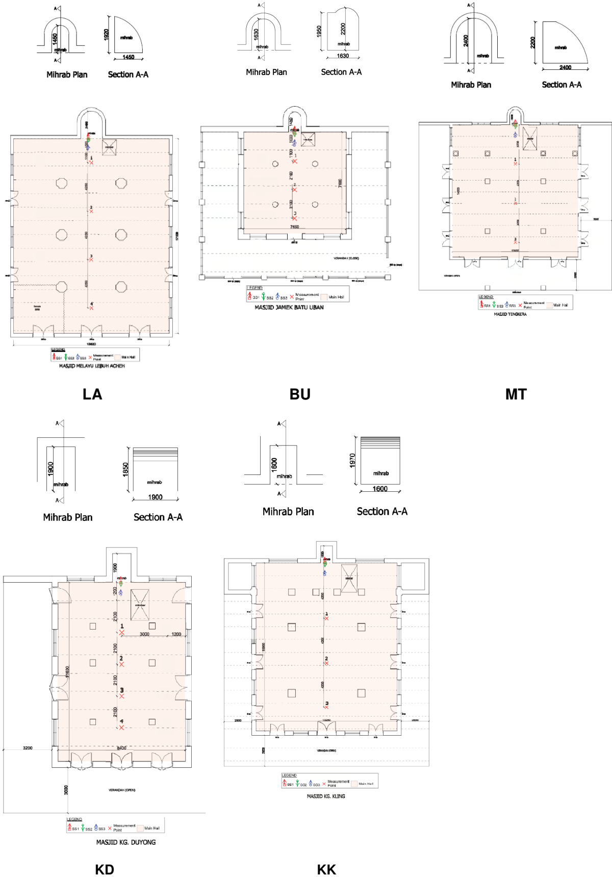
Figure1: Plan layouts with measurement points location, mihrab plans and sections
