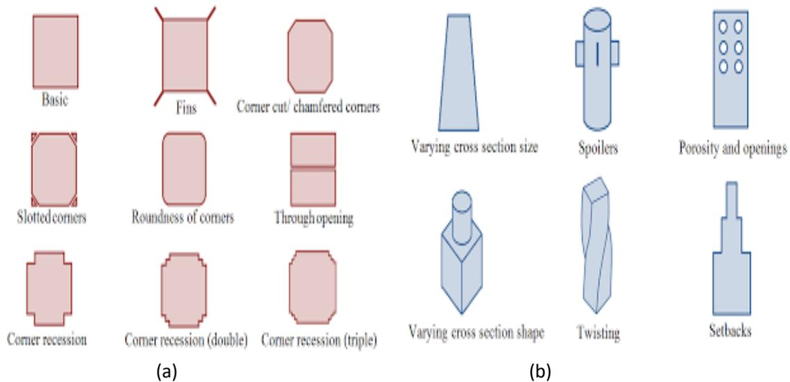
Figure 2: (a) Minor aerodynamic modifications; (b) Major aerodynamic modifications (Power & Jayachandran, 2019)
