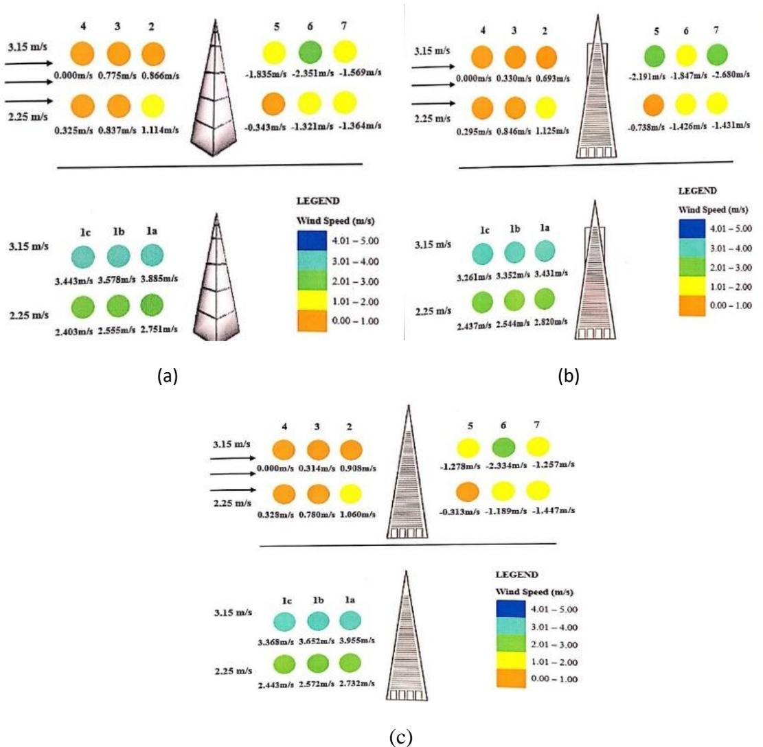
Figure 9: (a) Wind flow pattern of pyramidal model; above: wind flow from windward to leeward, below: wind flow from side surface; (b) Wind flow pattern of Transamerica model (section X); above: wind flow from windward to leeward, below: wind flow from side surface; (c) Wind flow pattern of Transamerica model (section Y); above: wind flow from windward to leeward, below: wind flow from side surface
