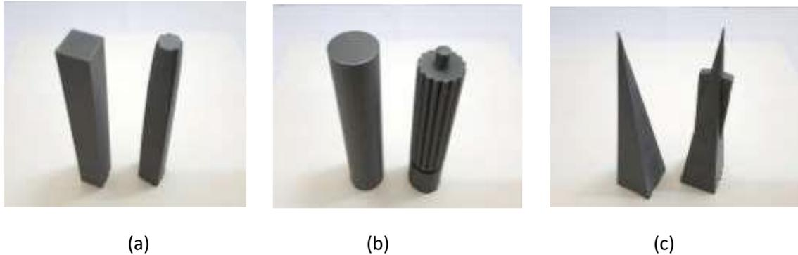
*Figure 3: (a) Square geometry and duplicated model of Gran Torre Santiago; (b) Cylinder geometry and duplicated model of Marina City Towers; (c) Pyramidal geometry and duplicated model of Transamerica*
