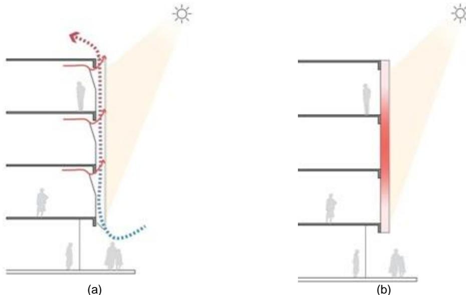
Figure 1. Comparison of heat mechanism in the DSF. (a) DSF in hot climate countries. (b) DSF in cold climate countries (Souza, 2022).
