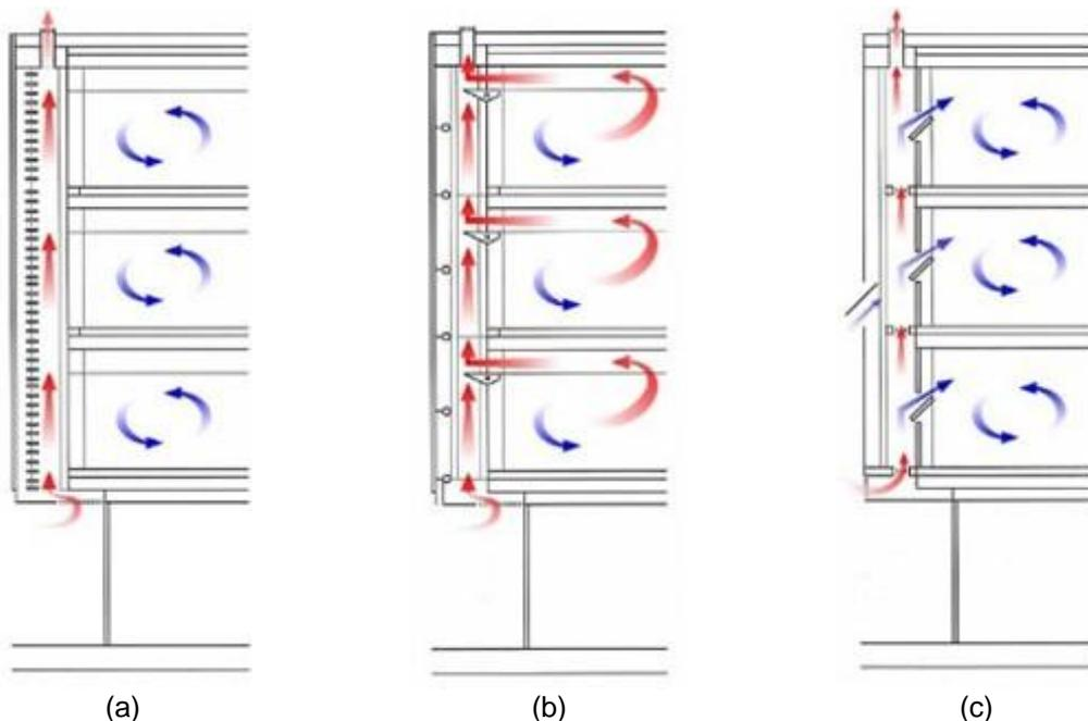
Figure 3. Type of DSF. (a) Buffer façade system (b) Extract-Air Façade System (c) Twin Face System (Boake, 2003).
