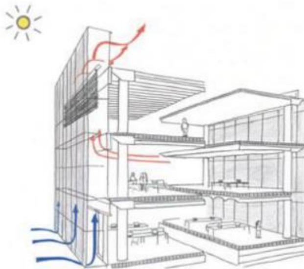
Figure 6: Double Skin Façade and Chimney.
